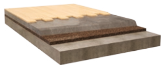
FLOATING SLAB WITH WOOD FLOORING
