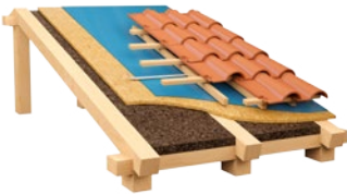
PITCHED ROOF WITH INTERNAL INSULATION BETWEEN RAFTERS
