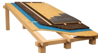
PITCHED ROOF WITH ABOVE RAFTER INSULATION
