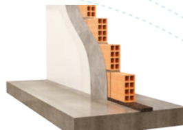
MASONRY WALL AND SLAB DISCONTINUITY
