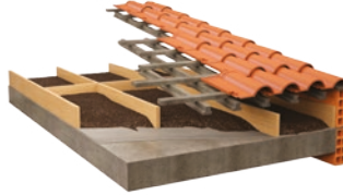
PITCHED ROOF WITH LOOSE FILL INSULATION BETWEEN JOISTS
