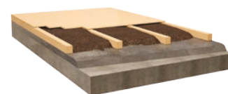
BETWEEN JOISTS LOOSE FILL
