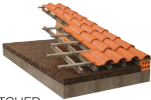
PITCHED ROOF WITH RIGID INSULATION OVER SLAB
